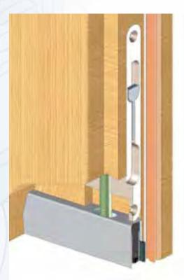
Maximum length = 1550 mm Minimum length with a deadbolt feedthrough 45 mm pin length = 335 mm
