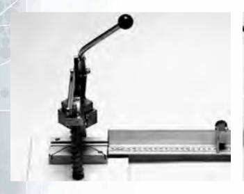
The DSV 4 die cutter is used for cutting sealing profiles to length and mitring the ends. The sealing profiles are then welded using the DSG 4 welding device.
